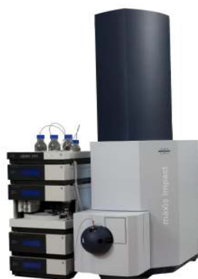
Figure 7: Mass spectrometry. Samples were analysed using a MaXis (Bruker Daltonics, Bremen, Germany) time of flight (TOF) mass spectrometer. Samples were introduced to the mass spectrometer via a Dionex Ultimate 3000 autosampler and uHPLC pump and variable wavelength detector. Ultrahigh performance liquid chromatography was performed using a Waters UPLC BEH C18 (50 mm x 2.1 mm 1.7 \mu m) column with 4 UV wavelengths selected. Gradient elution from 5% acetonitrile (0.2% formic acid) to 100% acetonitrile (0.2% formic acid) was performed in ten minutes at a flow rate of 0.6 ml/min. High resolution positive ion electrospray ionisation mass spectra were recorded
